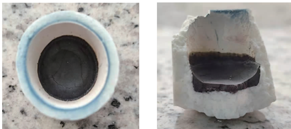
图 5 0.5 g 纯铁+0.2 g 样品+0.2 g 锡粒+1.6 g 钨粒熔样正面、剖面图 Figure 5 Front and profile of molten sample under the condition of 0.5 g iron+0.2 g sample+0.2 g tin granules+1.6 g tungsten flux.
